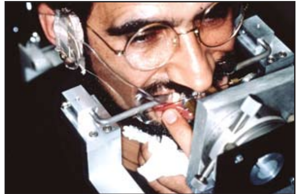
Fig. 7 In vivo friction test. 6 Maxilla is fixed in custom-cast splint, leaving mandible free. Testing machine pulls straight wire with preadjusted angulation and inclination through bracket on central incisor of spaced dentition. Whenever patient occludes, friction is immediately and markedly reduced.
